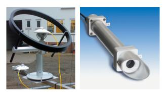
irradiance. The second sensor is covered from direct sun by means of a shadow ring or a tracked shadow ball. It measures the diffuse portion of global irradiance. The data logger **blueberry COMPACT** calculates in realtime direct irradiance as the difference between global and diffuse irradiance.
