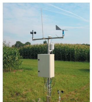
Measured data are recorded by the **blueberry COMPACT** data logger. The data logger sends measured data automatically via eMail. It provides realtime access via Internet.
