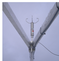
Fig. 3: Sonic anemometer, used as reference for most correlations
